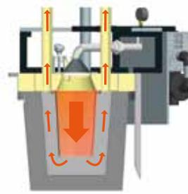
Functional principle of the ladle heating system
