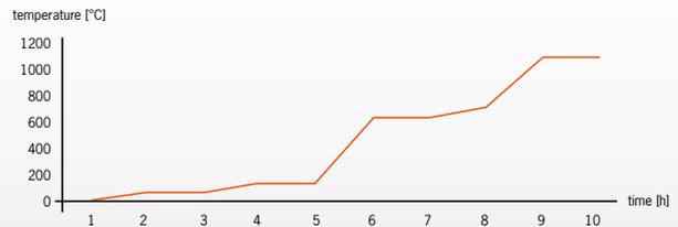
Drying Curve Refractory Concrete
